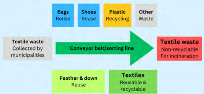
The set-up of UFF-Humana’s pre-sorting. The category ”Reusable & recyclable textiles” is sent for professional manual sorting in Europe.
